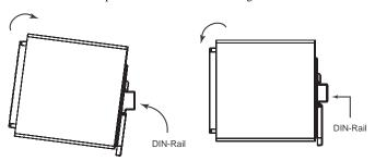
To remove the Moxa EDS-600 switch from the DIN-Rail, use a screwdriver to push down the spring-loaded bracket until it locks in place, as shown in the following diagram. Next, rotate the bottom of the switch upwards and then remove the switch from the DIN-Rail.
