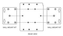
STEP 2—Mounting the EDS-600 on the wall requires 4 screws.
