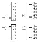
**STEP 1**: Insert the negative/positive DC wires into the V-/V+ terminals, respectively.
